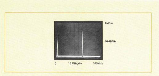
Figure 1.13 Display of a CW signal
