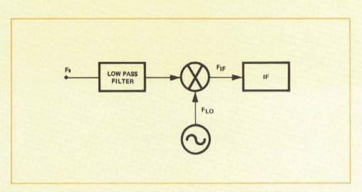
Figure 2.18 Low Frequency Analyzer Using Only 1<sup>-</sup> mode.
