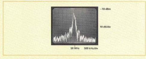
Figure 1.19 Jitter on a signal which is greater than the IF bandwidth.
