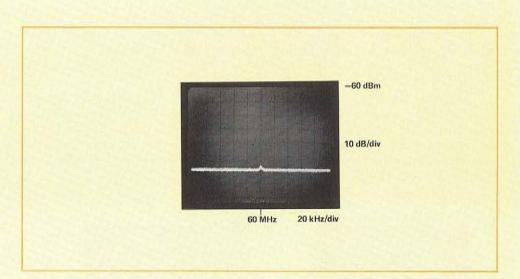
Figure 1.24 When signal power equals average noise power, the signal will appear 3 dB above the average noise level.
