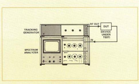
Figure 3.9 Swept Frequency Measurements.
