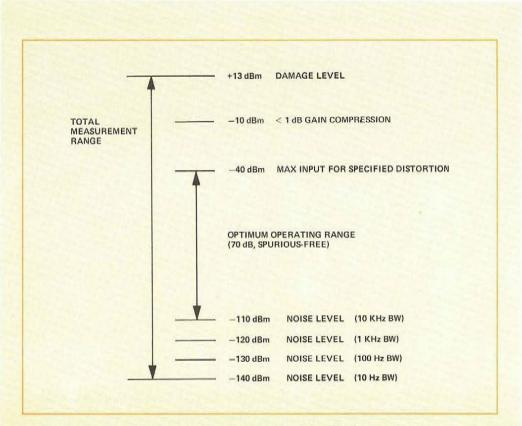
Figure 1.25 Typical spectrum analyzer display range.
