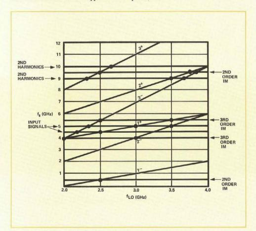
Figure 2.11 Spurious Responses to 4.5 and 5.0 GHz Inputs.
