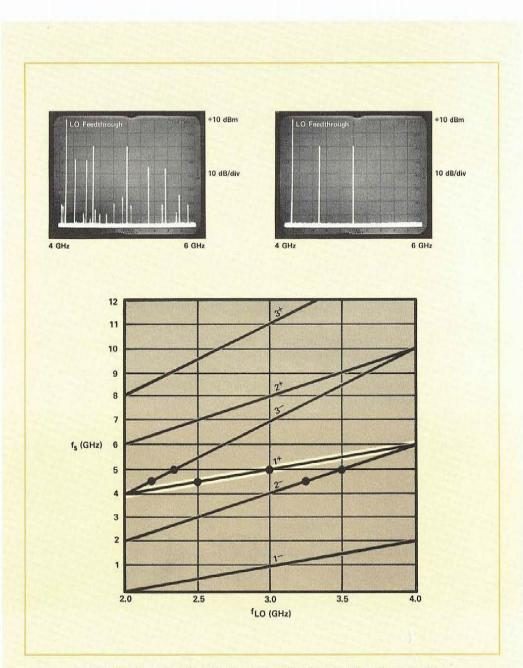
Figure 2.12 Elimination of Spurious Responses with Tracking Filter.
