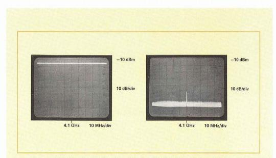
Figure 2.15 Elimination of IF Feedthrough with Preselector.
