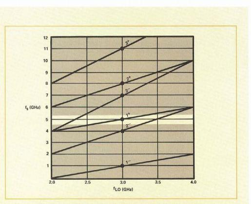
Figure 2.7 Rejection of Image Responses with Bandpass Filter.
