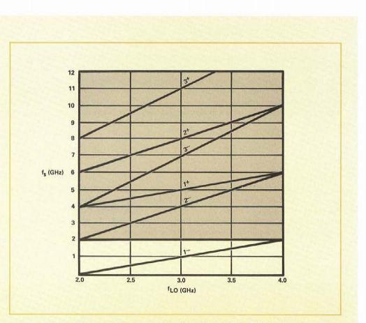
Figure 2.19 Only 1<sup>-</sup> mode is possible with Low Pass Filter at Input.
