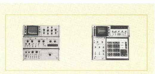
Figure 1.10 A multichannel and Fourier analyzer are shown on the left and right respectively. Both instruments are real-time spectrum analyzers.
