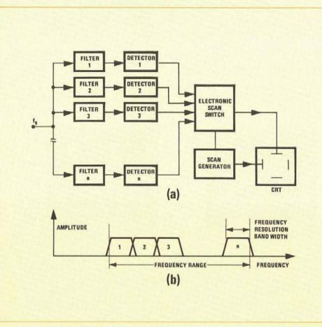
**Figure 1.9** (a) Block diagram of a real-time spectrum analyzer. The electronic scan switch samples the filters fast enough to display the instantaneous response of the input signals. (b) The bandpass filters are staggered to permit continuous coverage of the frequency spectrum.
