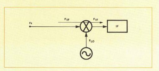
Figure 2.14 IF Feedthrough.
