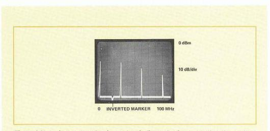
**Figure 1.14** An inverted marker is used to indicate the frequency that the analyzer is tuned to. The marker is only present in the full scan mode.
