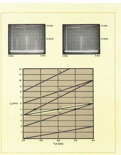
Figure 2.10 Rejection of Multiple Responses with Tracking Filter.
