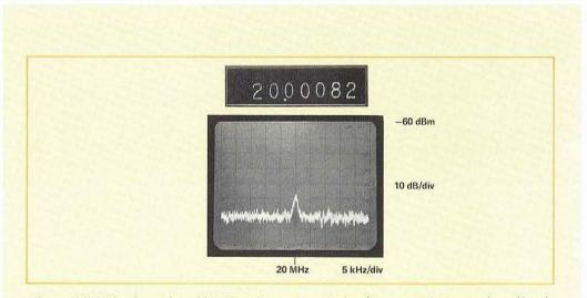
Figure 3.7 This signal is -110 dBm. It was counted using a spectrum analyzer/tracking generator.
