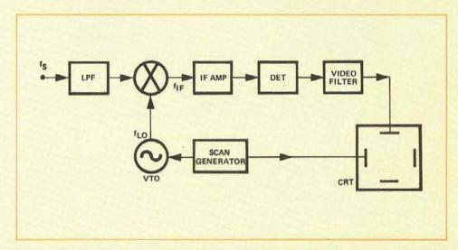
Figure 1.12 Block diagram of a swept superheterodyne spectrum analyzer. The input signal is mixed with a tuned LO frequency to produce a fixed IF which can be detected and displayed.
