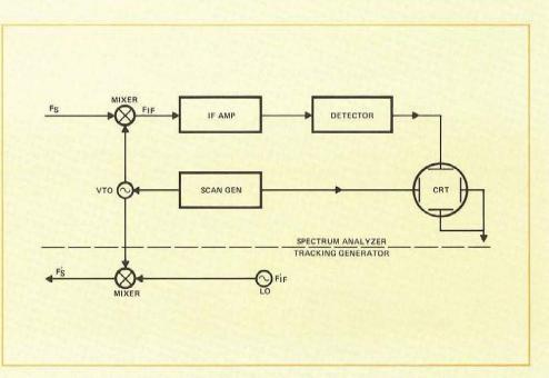
Figure 3.1 Simplified Spectrum Analyzer/Tracking Generator.
