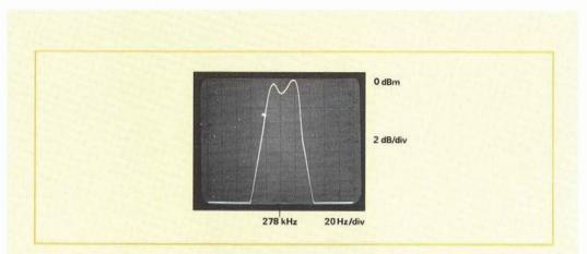
**Figure 3.11** Narrow and wide scanwidths of the spectrum analyzer/ tracking generator. The narrow scan width photo shows the passband details of the filter shown in Figure 3.10 on previous page.
