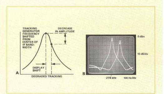
Figure 3.13 Degraded Tracking Effect.
