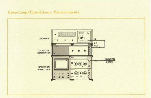
Figure 3.2 Open-Loop Configuration.
