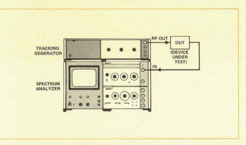
Figure 3.3 Closed-Loop Configuration.
