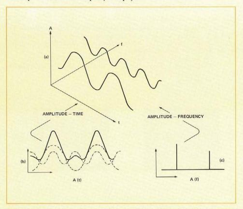
**Figure 1.1** Relationship between the time and frequency domains: (a) Three-dimensional coordinates showing time, frequency, and amplitude. The addition of a fundamental and its second harmonic is shown as an example. (b) View seen in the time domain. On an oscilloscope, only the composite  $f_1 + 2F_1$  would be seen. (c) View seen in the frequency domain. The components of the composite signal are clearly seen here.
