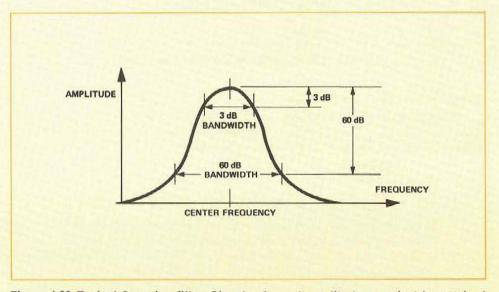
**Figure 1.20** Typical Gaussian filter. Signals of equal amplitudes can just be resolved when they are separated by the 3 dB bandwidth. Unequal signals can be resolved if they are separated by greater than half the bandwidth at the amplitude difference between them.
