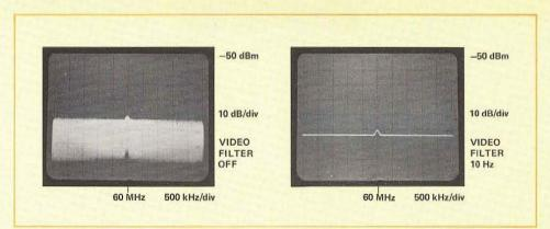
Figure 1.23 How video filter averages noise (right photo) for a better signal-to-noise ratio. No video filtering is used in the left photo.
