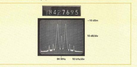
Figure 3.8 This is a suppressed carrier spectrum. The carrier frequency was counted as shown. Notice the selectivity of the spectrum analyzer/tracking generator system.
