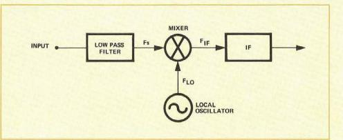
Figure 2.1 Spectrum analyzer Block Diagram.
