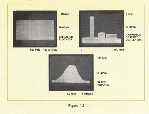
5. The swept frequency response of a filter or amplifier and the swept distortion measurement of a tuned oscillator are examples of swept frequency measurements possible with a spectrum analyzer, as shown in Figure 1.7. These measurements are simplified by using a variable persistence display or a tracking generator which will be described later.
